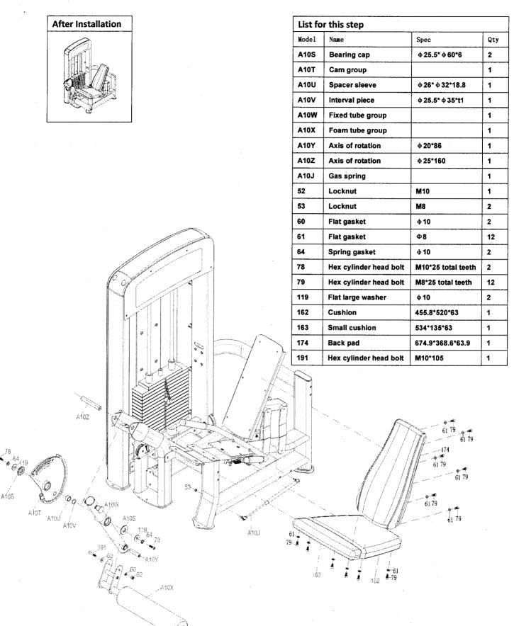
Step 4 Pulley installation diagram:
