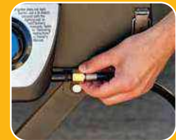
ATTACH ADAPTER TO GRIDDLE FUEL SUPPLY CONNECTION AND TURN BY HAND UNTIL TIGHTENED
