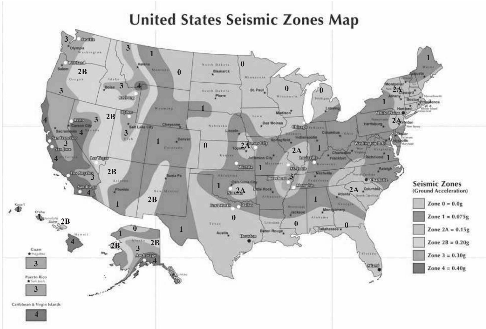
Mason-Lite Fireplaces have been tested and passed the seismic requirements for Modular Masonry Fireplaces throughout the entire United States. We understand that not every installation needs the extra security that is involved in a high seismic zones. Rebar is **ONLY REQUIRED** in Mason-Lite units in seismic zones 3 & 4 shown in the map below. We will supply rebar to all fireplaces shipped to in the United States unless otherwise requested.
