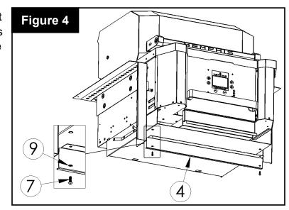
**Step 5)** Attach front lower caps (Part 5) onto the bottom corners of the grill using 4 screws (Part 7) and 4 washers (Part 9) (**See Figure 5**).
