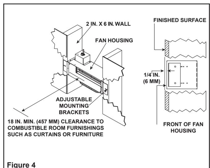
**Note:** If the fan housing is installed in a 2 x 4 wall, the front of the housing will protrude approximately 1/2 in. (13 mm) out of the wall without the drywall template. See Figure 5.
