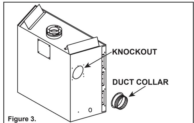
3. Determine the location for the air register/fan housing assembly. Cut a 5 in. x 13-5/8 in. (127 mm x 346 mm) hole between framing members (wall studs or floor joists). The fan and electrical connections must be accessible for servicing per local code requirements.
