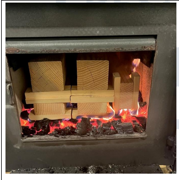
Test Fuel Loaded in Stove
