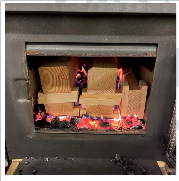
Test Fuel Loaded in Stove
