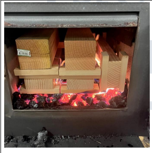
Test Fuel Loaded in Stove
