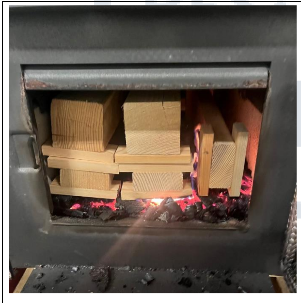
Test Fuel Loaded in Stove
