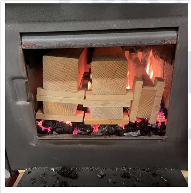
Test Fuel Loaded in Stove
