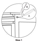
Attach wall mount to the product Find the 2 holes on the backside of the product. They are located on the top left and top right corners of the product. Securely install Part A and Part B in each hole. Tighten with Part E.
