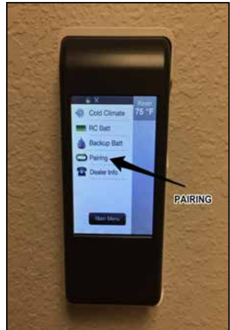
Figure 4.12 IFT-RC400 Wall Mount / Pairing Screen
