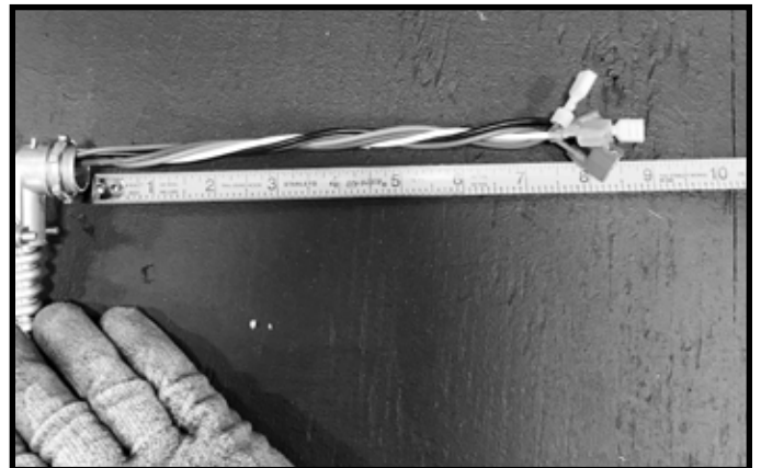
Figure 3.9 Sufficient Wire Extending Through Bracket
