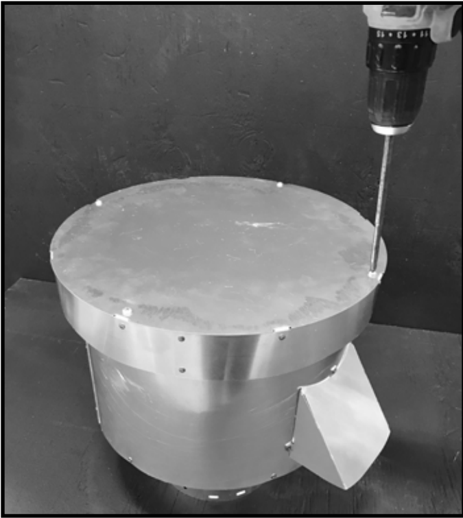
Figure 3.6 Remove Top Cap Screws
