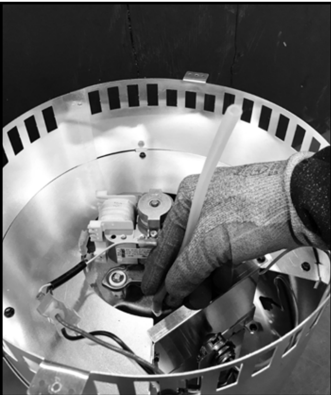
Figure 5.5 Remove Teflon Tubing from Blower
