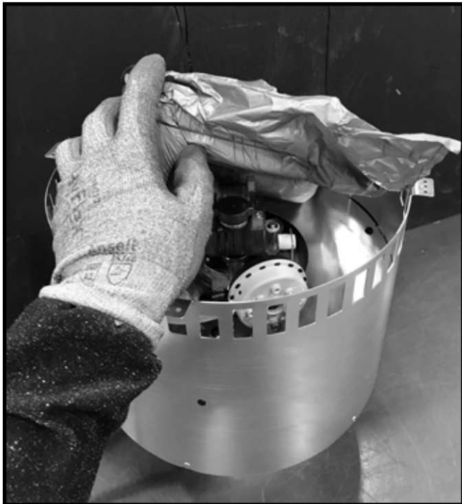
Figure 3.7 Remove Shipping Support Foam
