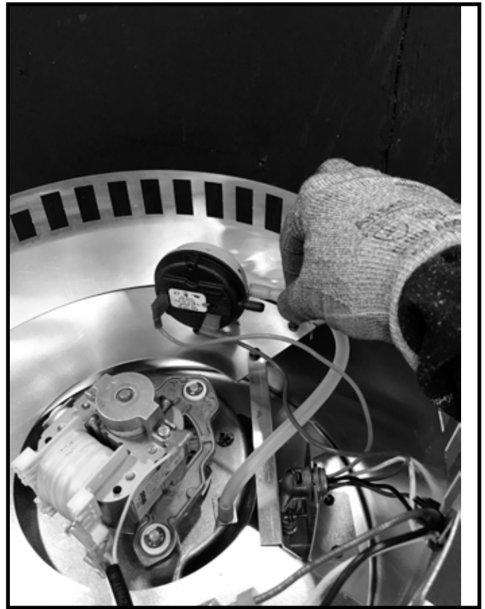
Figure 5.2 Remove Teflon Tubing
