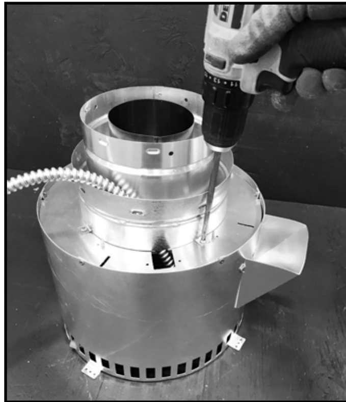
Figure 3.11 Attach Starting Collar
