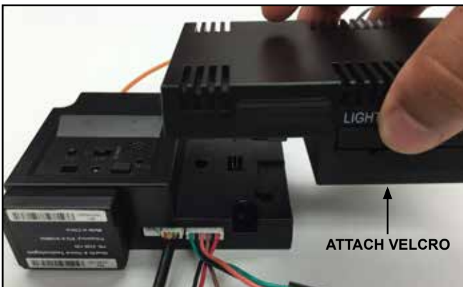
Figure 4.3 Connecting IFT-ACM and IFT-ECM
