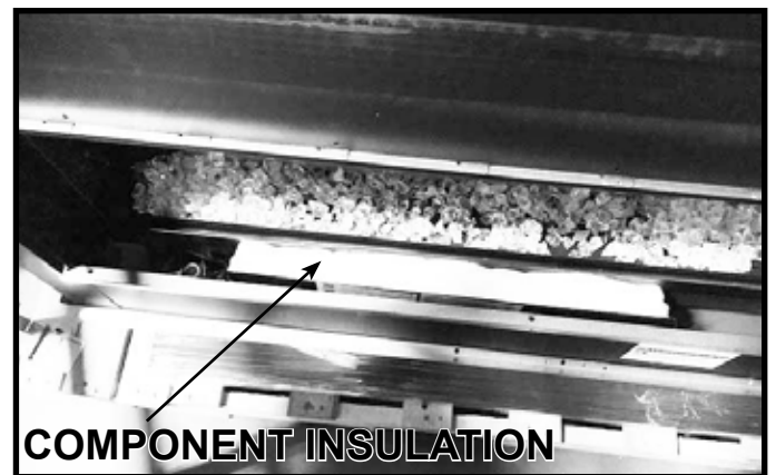
Figure 11.3 Component Insulation Location
