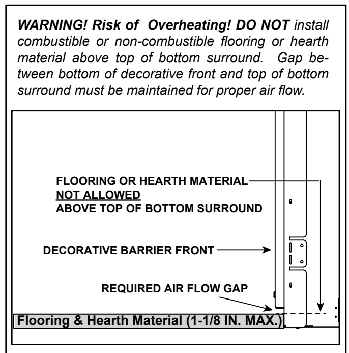
Figure 10.3 Required Air Flow Gap
