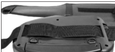
4.3.3 Make the fastening belt pass through the respiratory system's 2 belt loops.
