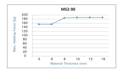
Material used in the magnet is N35H, Safe operation tempreture ≤120°C;
