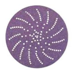
The 3M™ Cubitron™ II Sanding Disc is a revolutionary advancement in abrasive technology featuring triangular shaped ceramic mineral. As the triangular shaped grain wears, it continually fractures to form sharp points that slice through the substrate, wear evenly and provide extra-long life and consistency
