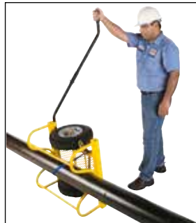
2. Use ratchet to flip Cricket and pipe
