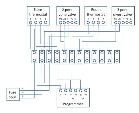
The following control wiring diagrams ensure that the district heating system is isolated from the dwelling when charging is not required.
