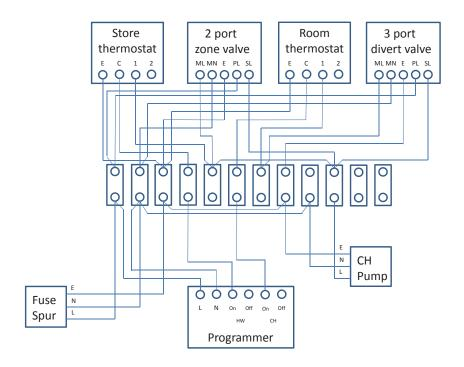
Wiring diagram – HW & CH pump required
