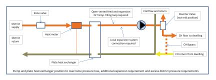
In this instance, the plate heat exchanger provides a full pressure break between the district heating system and the dwelling system. The dwelling system will need to cater for expansion and circulation requirements. This may be used where excessive district heating pressure occurs.
