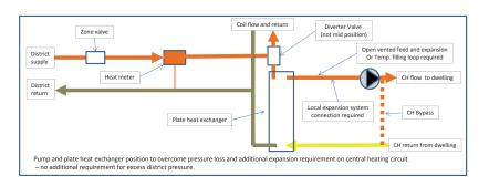
Here, the plate heat exchanger has been fitted because the expansion requirements of the central heating system are to be handled in the dwelling rather than the whole system, or the components in the central heating system are not capable of withstanding the pressure of the district heating system.
