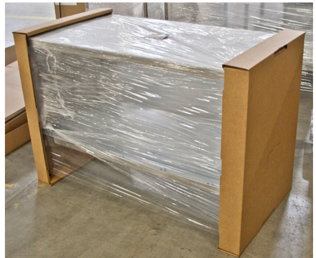
Fig. 2: Wrapped Table with End Caps
