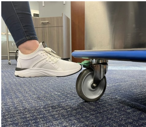
Fig. 25: Lift up caster lock with foot
