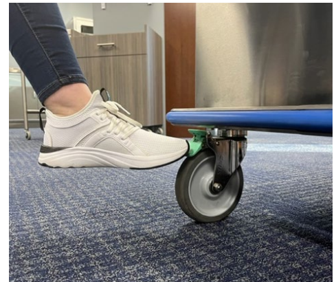
Fig. 26: Push down caster lock with foot
