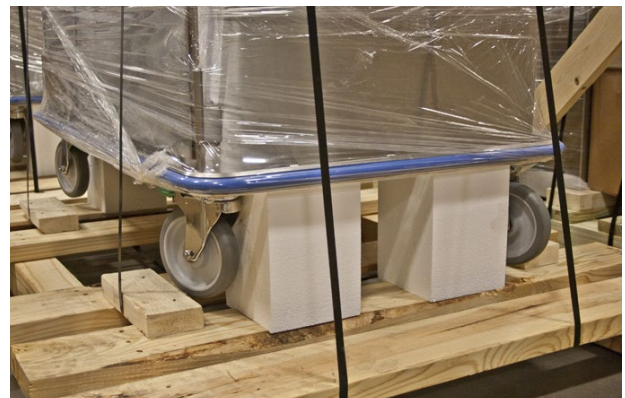
Fig. 2: Foam Blocks Protecting Casters
