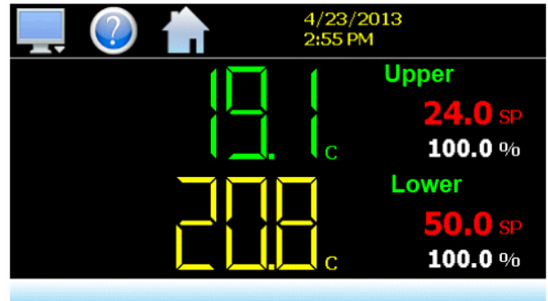
Fig. 42: Dual Chamber Temperatures and Set Points
