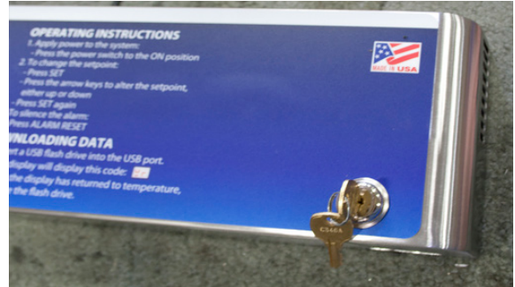
Fig. 159: Overlay-Cam Lock Location - Left Hinged Door
