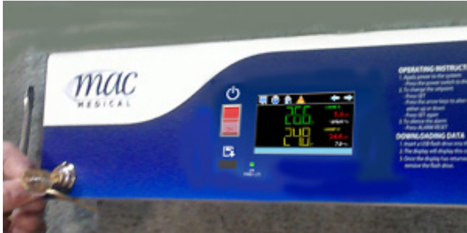
Fig. 158: Overlay - Cam Lock Location - Right Hinged Door
