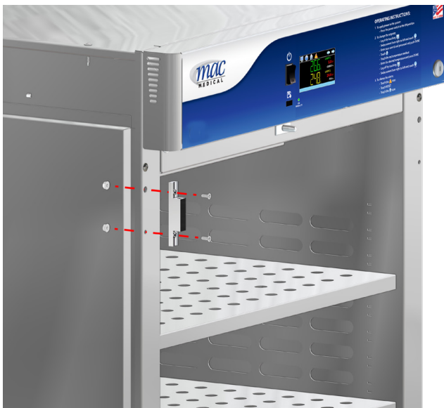
Fig. 172: Install Male Hinge Halves in New Position
