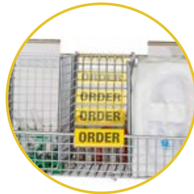
When front bin is empty, user moves flipper down signaling need to re-stock / re-order
