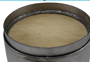
1. Welded extension ring creates alignment problems
