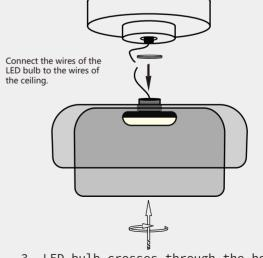
3. LED bulb crosses through the hole of the first large shade then with the third gasket tightened.
