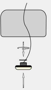
Put the gasket on the LED bulb then tighten it.
