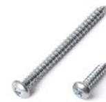
Fastening screws High quality wood screws are sufficient for fixing the grates to a timber joist structure. However with the Ryno aluminium substructure, stainless steel screws should be used to ensure no corrosion occurs.
