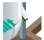
**7.2** Pull back the breather membrane on the product and carefully cut away the rest of the insulation, leaving just the grey membrane in the valley.
