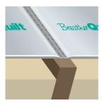
**1.2** Begin the next roll from this rafter, by butt-jointing it to the end of the first roll and staple in place.
