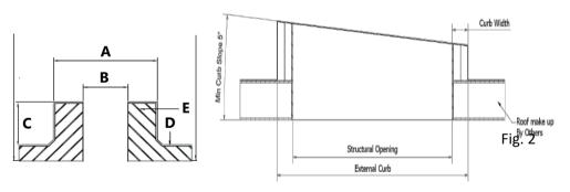
This will provide for a maximum waterproofing thickness of 15mm all arou Note: for asphalt in excess of 13mm thick, contact your supplier.
