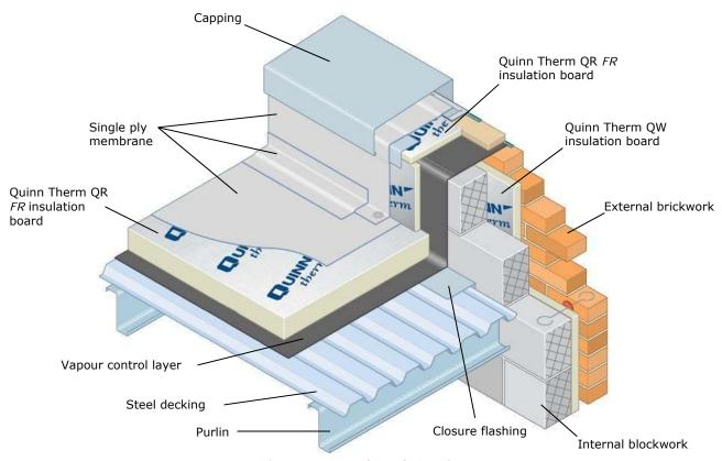
Figure 1: Metal Deck Roof
