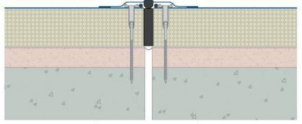
Figure 8: Movement Joint
