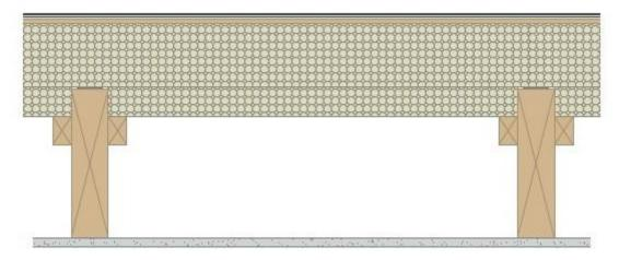
Figure 1: Insulation between joists
