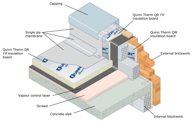
Figure 5: Concrete Deck Roof
