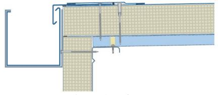
Figure 4: Eaves Gutter
