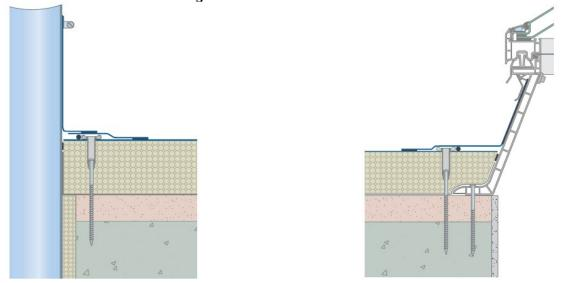
Figure 6: Pipe Penetration
