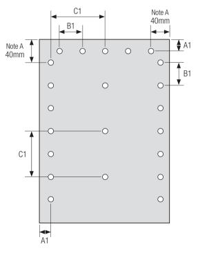
Note A: The first fixing in from the corner for both horizontal and vertical fixing must be 40mm in from the edge.
