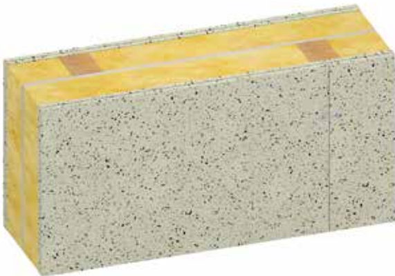
EL 120: Timber stud partition with 2 layers of mineral wool insulation (min density of 28kg/m 3 ) – 120 minutes fire resistance.
