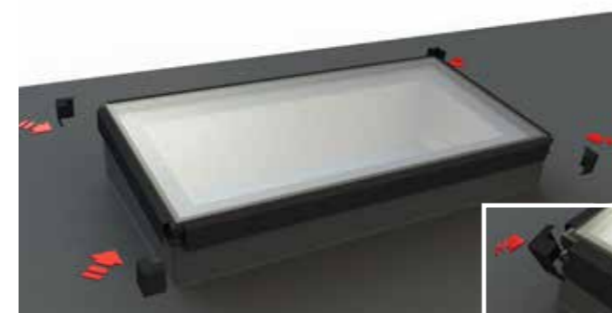
5 Fit the corner trims by hooking them under the external claddings and rotating them over, clipping them into place.
