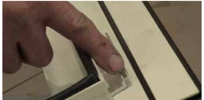
10 The hinge channel fits over the outer frame hinge.
