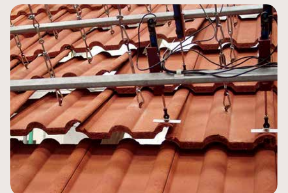
REDLAND SEVERE LOAD TESTING FACILITY
