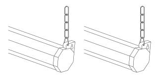
1) Pull the screen down from the lanyard or from the handle only in a 90-degree angle. Do not attempt to pull the screen down by the surface or touch the screen, as it will damage the screen and void the warranty.
