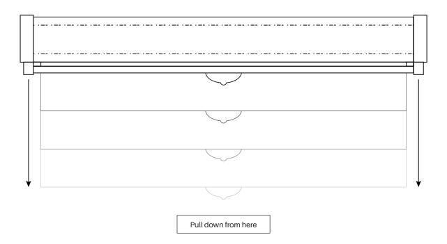
**Note:** Improperly bringing the screen up/down will damage the screen material or rolling system. RETRACTION TIP: If you are not able to pull the screen down two inches when attempting to retract it, give the screen a quick yank downwards with a little bit of force. Please be sure to not stand directly under the housing of the unit when yanking down on the screen.
