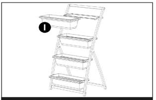
8. Place plastic planters ( G ) onto the planter hangers. For cascading drainage make sure planter holes are facing frontward.
