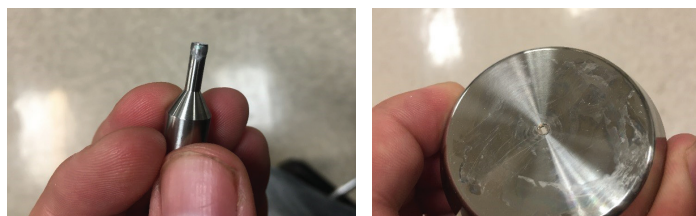
Figure 1: The MicromATR Vision press tip and diamond ATR puck after measuring a methanol cast film on the ATR. Both parts are easily removed for convenient cleaning, inspection, or for trace sample placement using a stereo microscope.
