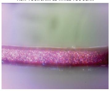
**Figure 1:** Image of wire insulation on MicromATR Vision through the diamond ATR.
