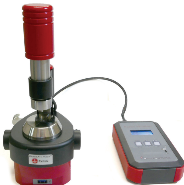
Figure 1: MicromATR Q with digital force readout
