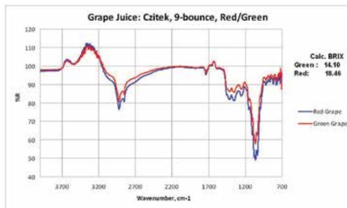
**Figure 1:** Spectrum of fresh grape juice from a squeezed grape - 9 reflection Cleartran ATR head
