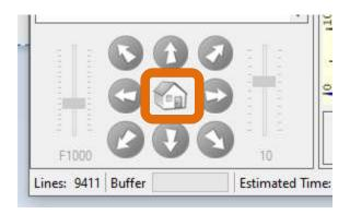
After homing has completed use the arrows at the bottom left of the screen to move the laser to the bottom left of your material.
