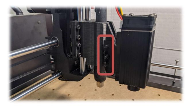
Slide the Laser onto the 3 Bolts of the ZAxis. Attach the provided wingnut on the center bolt.
