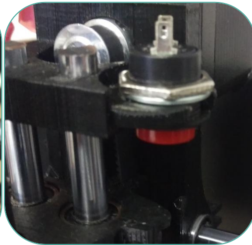
Y Axis (This End Stop switch comes pre wired)
