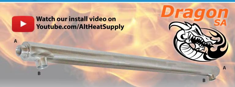
High Quality Fin-Enhanced Sidearm Heat Exchangers are designed with the natural thermo-siphon concept on the domestic hot water side. Made of 304 stainless steel, fin-enhanced sidearms increase heat transfer efficiency significantly by using a finned tube internally, which has a surface area five to eight times bigger than bare tube and produces greater turbulence on the system side.
