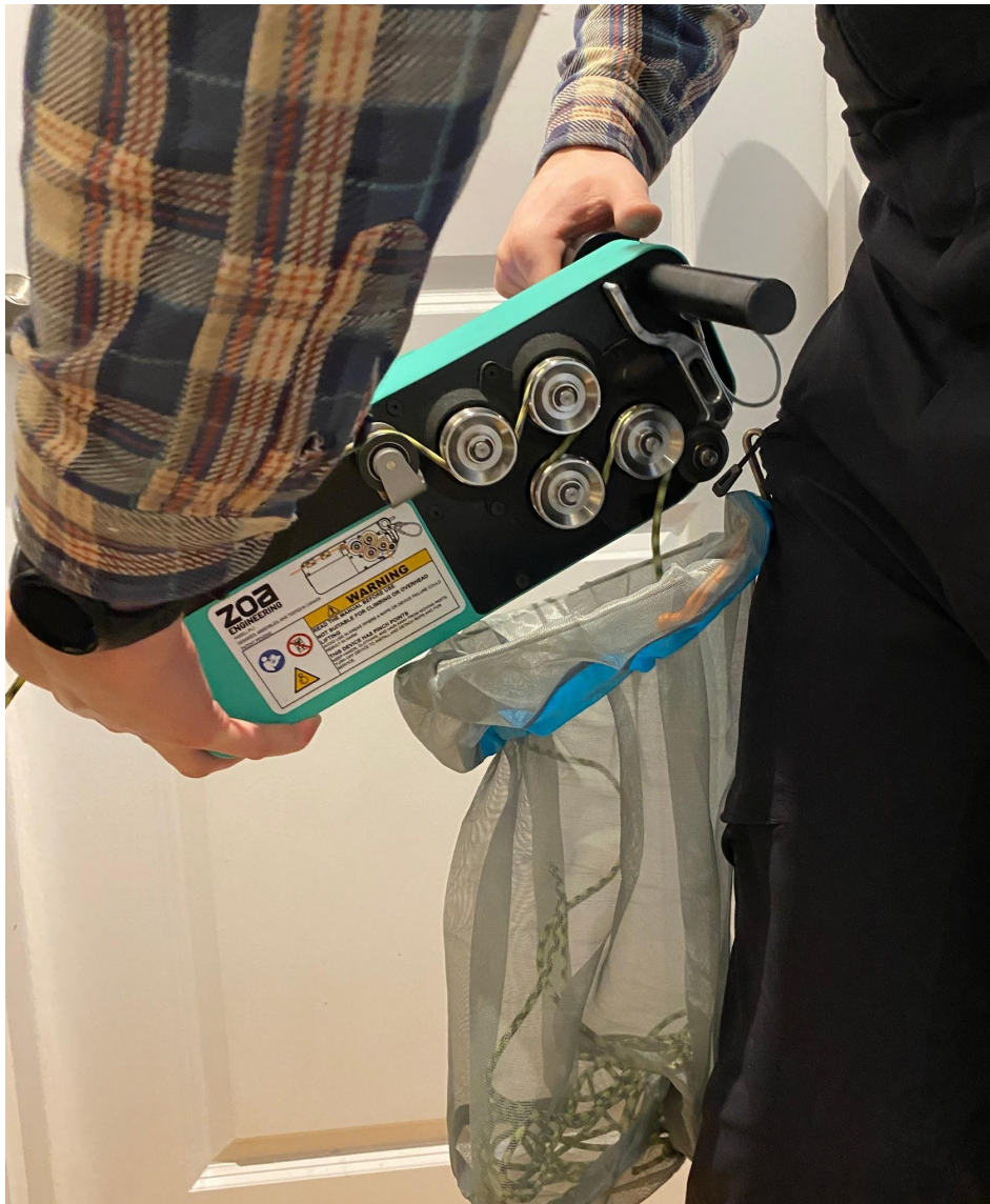
Figure 10. Flake rope into bag using the PL1 as shown, compressing rope when necessary
