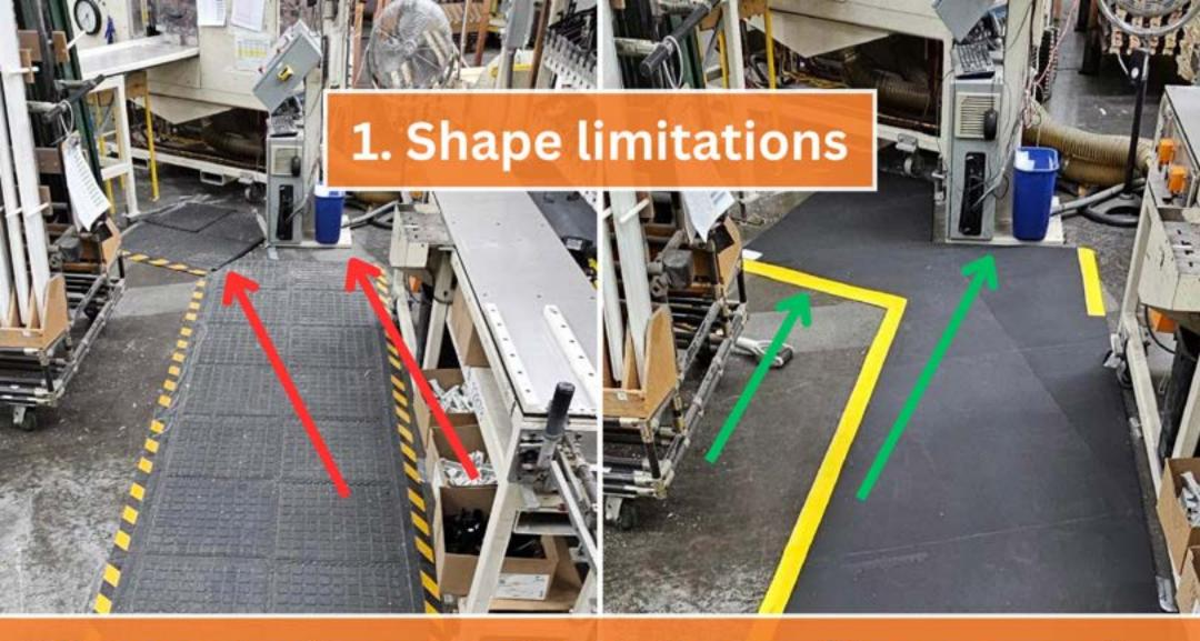
Tiles can be "snapped" together to fit an array of custom layouts. However, they are square which limits you to 90-degree configurations. As a result, the tiles above had to be manually cut and laid next to each other to fit the area. <a href="Trip hazard">Trip hazard</a>. The custom anti-fatigue mat was designed with multiple angles to seamlessly fit the workstation.
