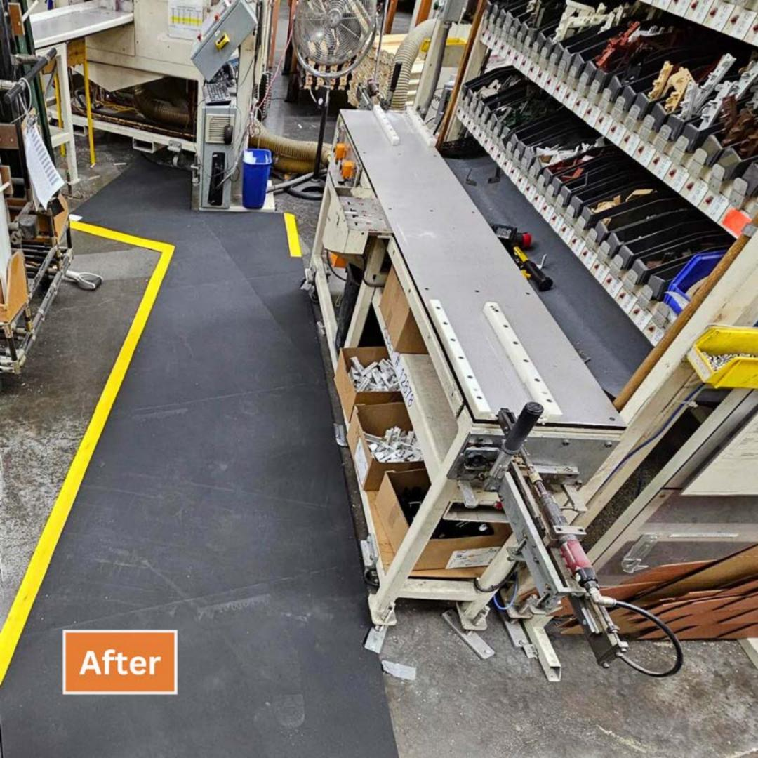
Tiles are made from plastic material. It's versatile but not impervious to liquids or chemicals. In environments with accumulation, particles and chemicals embed in the seams and pull the tiles apart. Trip hazard. On the right, the custom mat is made from 100% nitrile, which is impervious to liquids, chemicals, and particles; it also never flattens, providing critical ergonomic support.
