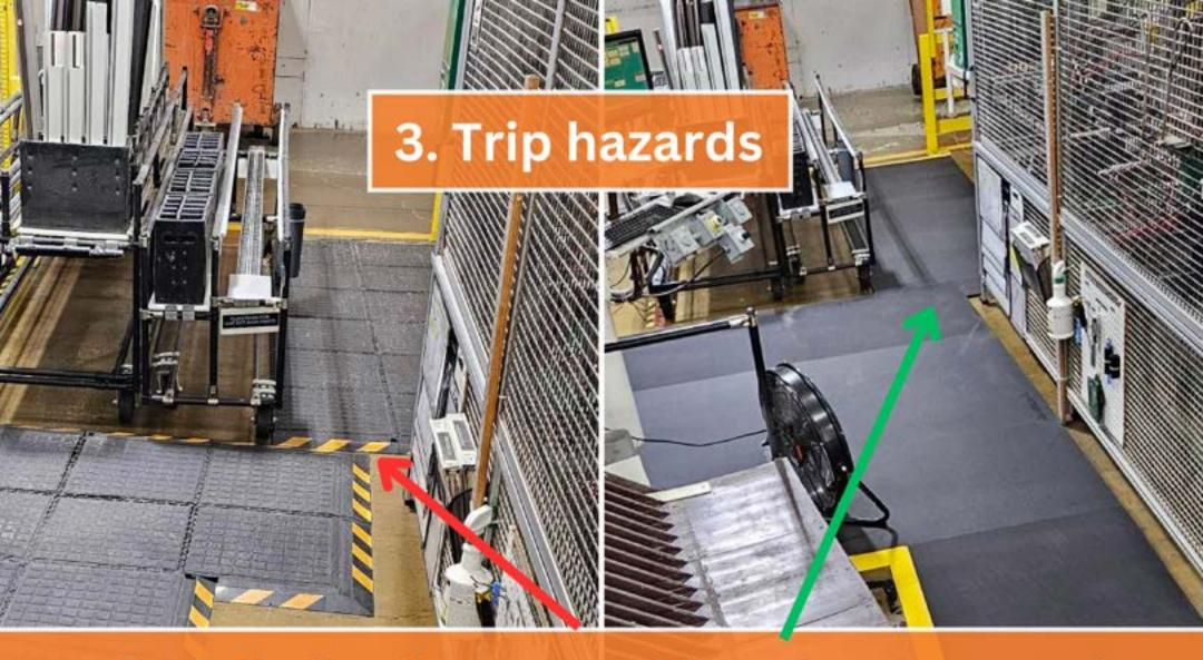
On the left, the tiles are unable to be connected through the small gap between equipment. So, they're placed next to each other. <u>Trip hazard</u>. On the right, with the ability to be designed to "any shape and size," the custom mat fits seamlessly throughout the area; no gaps, on/off stepping, or inconsistent thicknesses.
