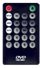
POWER (red) Switch DVD mode on/off EJECT (green) Ejects the DVD SETUP DVD mode settings MENU Opens the main menu GOTO Function key
