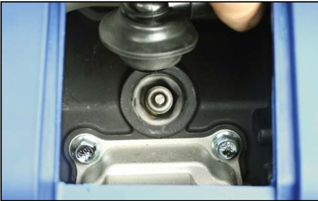
Figure 42 – Removing the Spark Plug Boot
