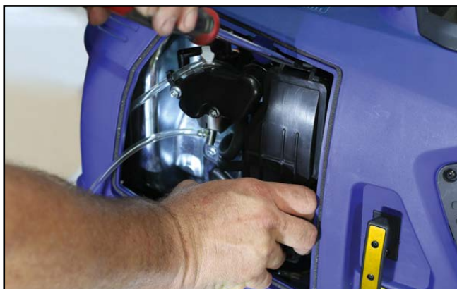
Figure 34 - iGen1200 Removing the Air Filter Cover
