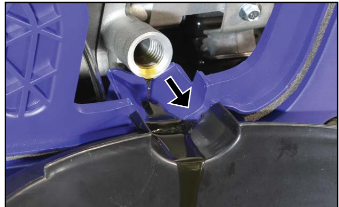
Figure 32 – Draining the Engine Oil
