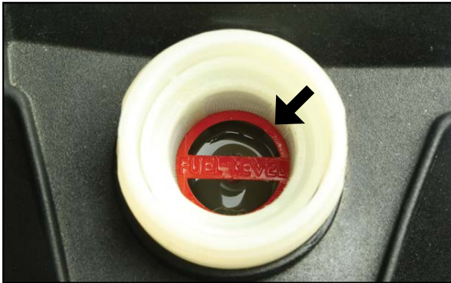
Figure 12 – Maximum Fuel Fill Level
