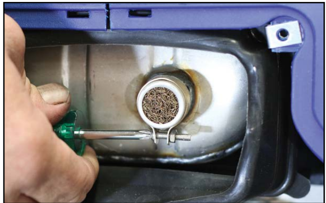
Figure 47 – Removing the Spark Arrester Band Clamp
