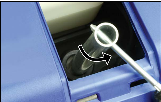
Figure 43 – Removing the Spark Plug
