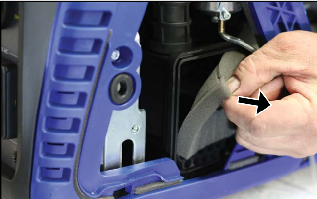
Figure 37 - Removing the Air Filter Element
