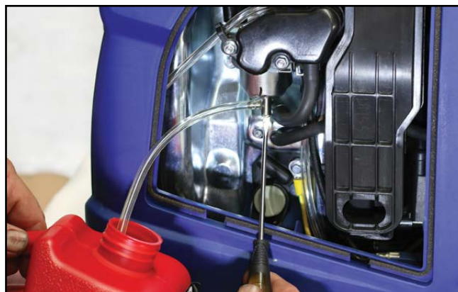
Figure 50 – iGen1200 Draining the Carburettor
