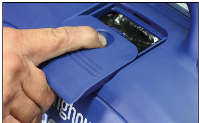
Figure 41 - iGen2200 & 2500 Removing the Spark Plug Access Cover
