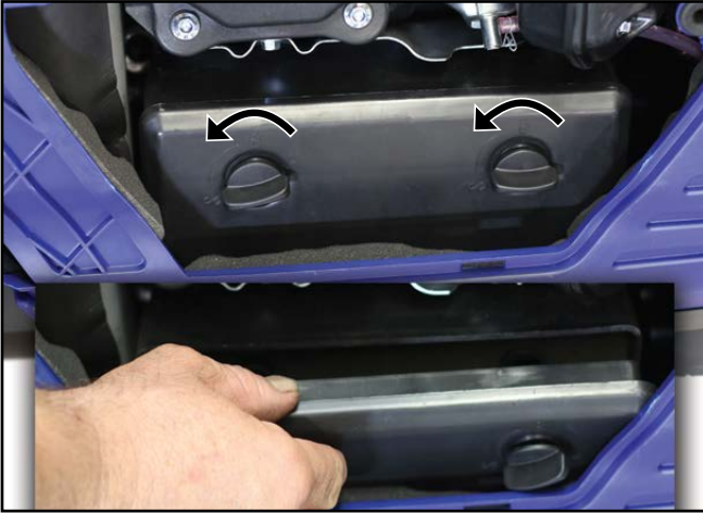
Figure 36 - iGen4500 Removing the Air Filter Cover
