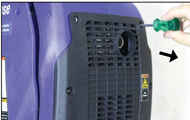
Figure 45 – iGen2200 & 2500 Removing the Muffler Access Cover
