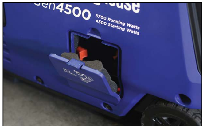
Figure 28 - iGen4500 Removing the Oil Access Cover
