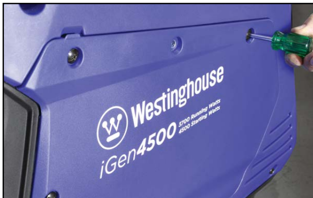
Figure 33 - iGen4500 Removing the Engine Access Cover
