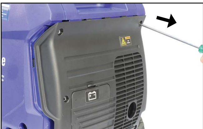
Figure 46 – iGen4500 Removing the Muffler Access Cover
