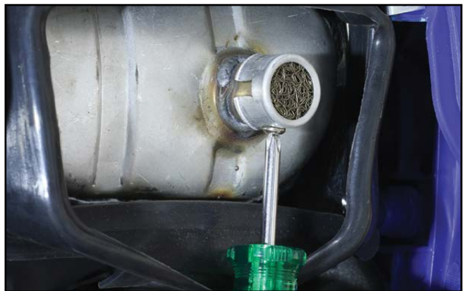
Figure 48 - Removing the Spark Arrester Collar and Screen
