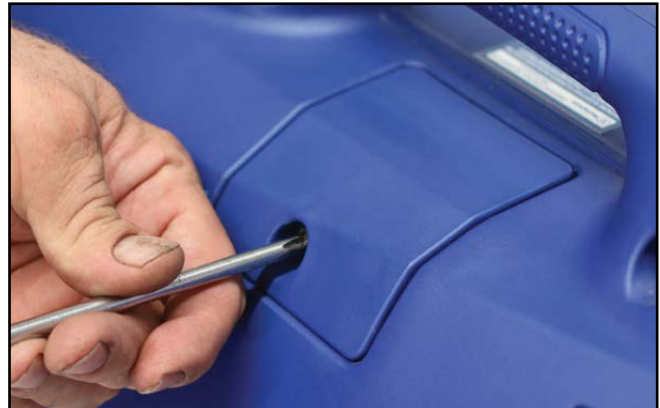
Figure 40 - iGen1200 Removing the Spark Plug Access Cover
