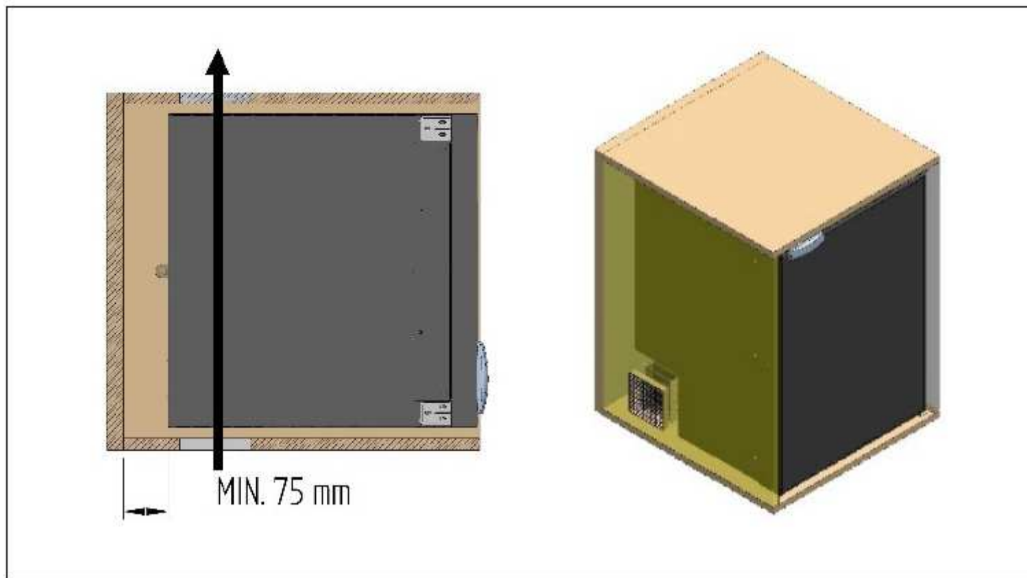
Image 3b – side hole and air flow
