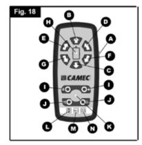
Straight forward (18B) Straight reverse (18C) Left forward (18D) Left reverse (18F) Right forward (18E) Right reverse (18G)
