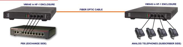
NOTE: The VMX4E & VMX4S multiplexer cards can also be installed in the HF-2SS and VMX20 chassis for rack-mount applications.
