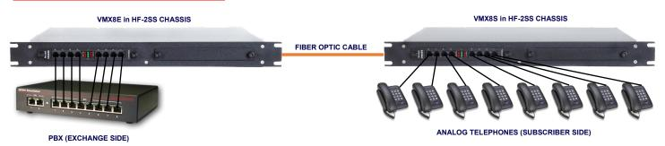
NOTE: The VMX8E & VMX8S multiplexer cards can also be installed in the HF-1 enclosure for standalone applications.
