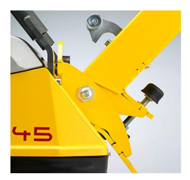
The particularly designed Wacker Neuson guide handle provides a hand-arm vibration of under 2,5 m/s<sup>2</sup>.
