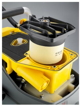
The pulled in air passes first through the cyclone filter where the majority of dirt particles are already removed. This is followed by the foam material prefilter. The pre-cleansed air only meets the main filter at the end of the process. This results in a manifold increase of the air filter's service life. In addition, there is only minimal loss of pressure. This ensures a consistently high engine performance.
