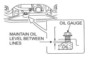
Figure 6. Vibrator Oil Gauge
