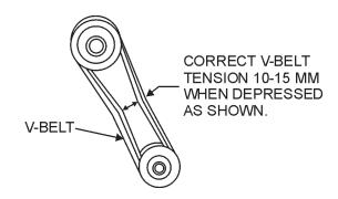
Figure 10. V-Belt Tension
