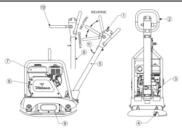
**Figure 2. Compactor Components**
