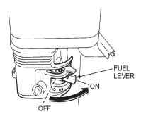
Figure 11. Fuel Valve Lever
