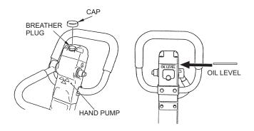
Figure 7. Hydraulic Oil Check
