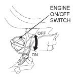
Figure 12. Engine ON/OFF Switch
