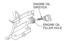
Figure 4. Engine Oil Dipstick
