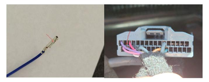
Note: Pin is fragile and can be damaged with improper installation. It is best to push the pin in firmly with a small flathead screwdriver or other fine tool. Double check the pin seated fully.
