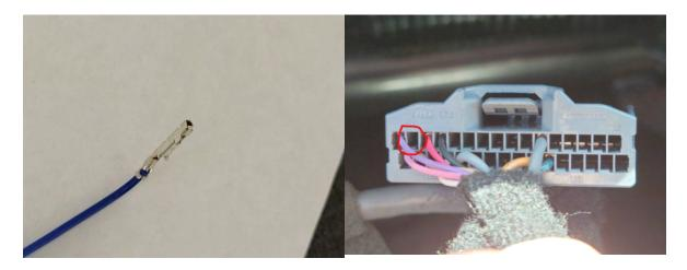
Note: Be sure to line up the protrusion on the reverse wire pin with the corresponding indent in connector C. The protrusion and the corresponding indent are shown below with red arrows.
