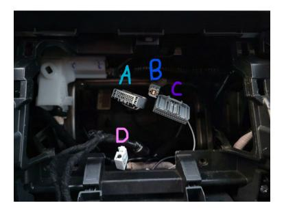
8. Now we start plugging things in. Double-Sided tape the GPS Antenna to this black part of the dashboard. The location below is an example. Connect the GPS Antenna connector to the back of the new head unit as shown.
