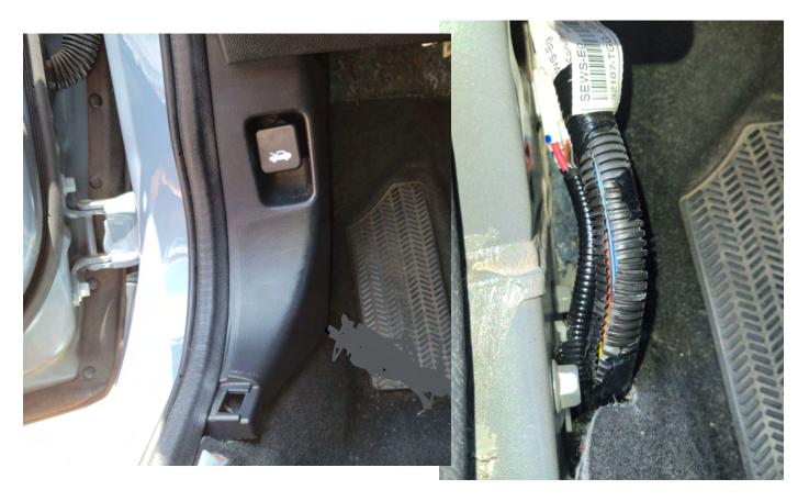
Under the plastic sheathing, you should be able to identify two mint green wires. One of these two wires is the correct one for our reverse signal. The plan is to try one wire to see if the reverse signal works, if not, then we can use the second wire.
