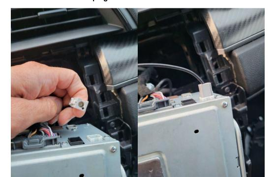
21. Now you can double sided tape the AM/FM Tuner in a location behind where the new head unit is going to be placed. The area circled in red is an example. It might be easier to remove the two metal brackets from the AM/FM Tuner if they are included with yours.
