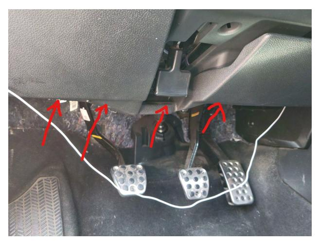
Reinstall drivers side kick panel and foot skid plate. Reverse wire installation is complete. If after powering the unit up and selecting reverse the camera does not show up, Remove the T-Tap connector and try the second mint green wire.
