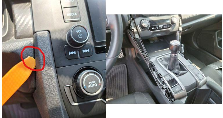
4. Pry up on the two circled tabs on the A/C control panel. A/C control panel should pop out and should allow you to disconnect the two connectors from the back of the panel.
