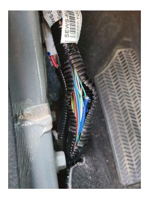
Use the included red T-Tap connector to tap into one of the mint green wires. Position the wire into the T-Tap as shown, and clamp the T-Tap together.
