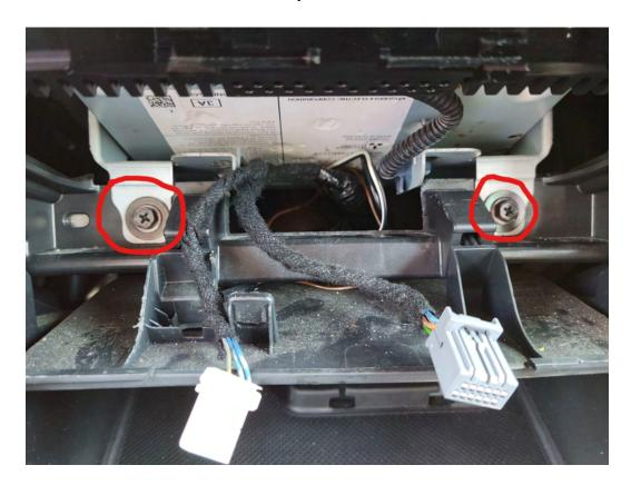
6. Pry up carefully on the headunit at the two circled points. You should hear a click or pop when you successfully pry up. At this point, you can pull the head unit out of the dashboard using the two points circled at the top of the head unit.
