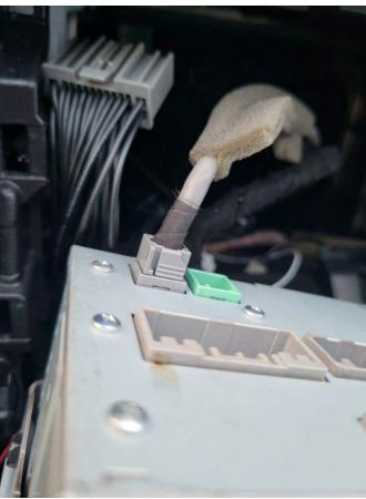
14. \*This step is only required for reverse camera functionality. What we are essentially doing is installing a wire into connector C, and routing the other end of that wire to the drivers side kick panel to pick up the reverse signal.
