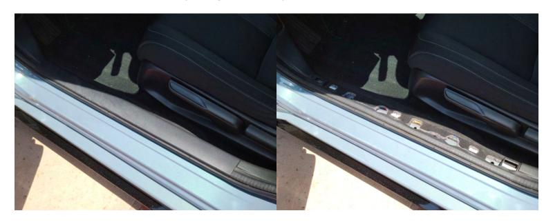
Remove the kick panel by pulling on it with your hands. You should see a loom of wires under some plastic sheathing.
