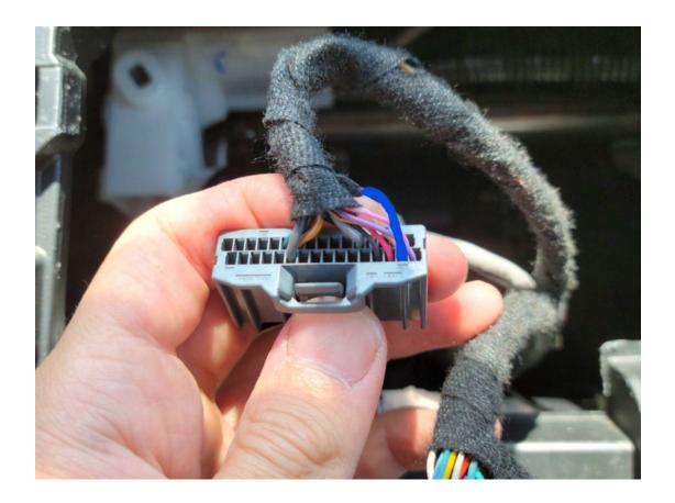
Now insert this connector C with the reverse wire installed into the back of the new head unit.
