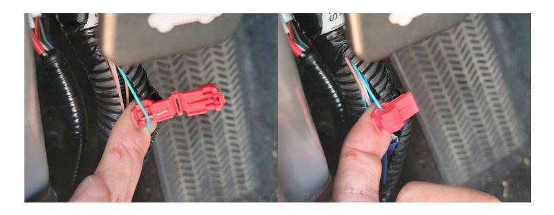
Once you have done this, you can connect the reverse wire spade connector to the T-Tap Connector.
